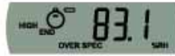
Highest reading of humidity sensor after logging has ended, upper alarm specification was exceeded battery ius low
