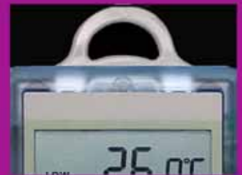
Moulded plastic lug allows logger to be hung from a hook or padlocked to an item.
