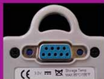
Download via the USB to Serial Port Adapter cable, no interface required.
